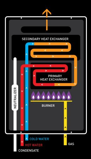
Developed to reduce wasted energy this unit pre-heats the water using heat from the gas exhaust, meaning you'll use less energy.
